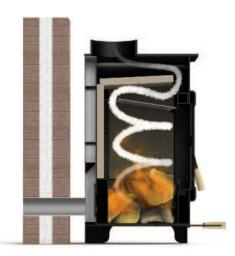
Where possible it always pays to room seal a stove. The average chimney will drag all the warm air from a room once every single hour. All models can be room sealed through an outside wall to completely eliminate this heat loss. This alone can add up to 50% efficiency.
